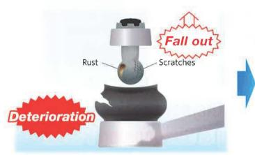
If the dust cover is broken, the ball stud is getting rusty and worn out.
